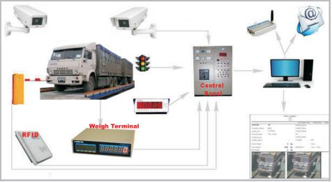
Automated Electronic Weighbridge System - Weigh Soft is a intelligent solution that turns your weighbridge to a simple unattended terminal, eliminating the need of weighbridge operator. The system can be customized with many add-ons like camera plate recognition, surveillance cameras, traffic barriers, traffic lights, etc. This innovative weighing application developed by **AMSTEL** is suitable for waste recycling plants, biomass to energy plants, oil and gas stations, cement plants etc.
